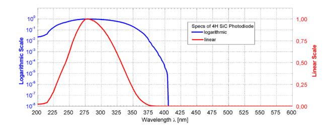
Broadband SiC based UV photodiode A = 1.00 mm<sup>2</sup>
